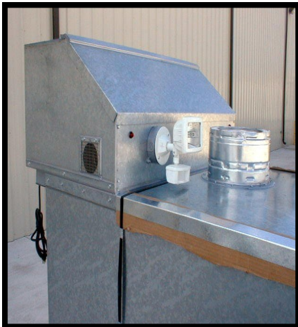
EXTERIOR COVERING BUILT FROM 1/16 INCH GALVNZED PLATE
