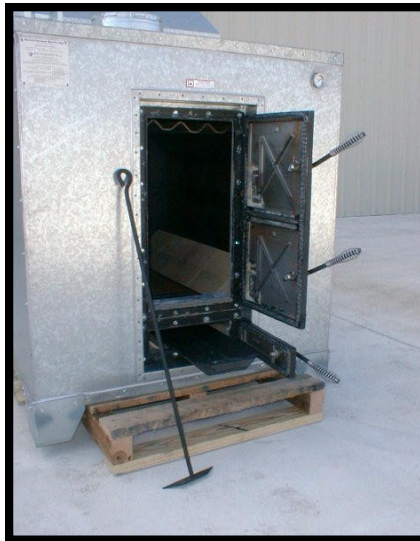
FIRE BOX BUILT FROM 3/16" STEEL PLATE, ALL WELDED CONSTRUCTION WITH CAST IRON GRATES
